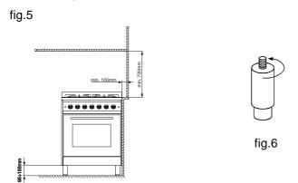
Prior to installing the cooker, the 95 - 155 mm high supporting feet (provided) should be fitted into the holes to be underneath the cooker (fig. 6). These feet are screwadjustable and whenever necessary should be used to make sure the cooker is level.
